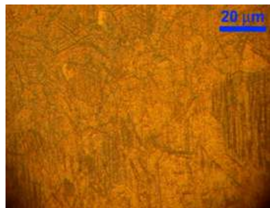
Figure 6. Sample(316)weldedprocess (TIG) ZACautogenouscross section(1000X).
