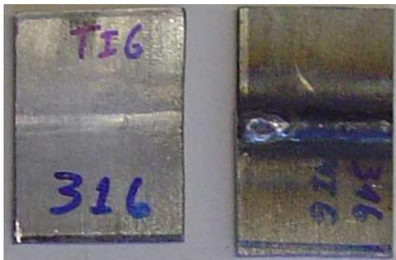
Figure 2. Aspects of the weld in TIG and MIG steels AISI 316.
