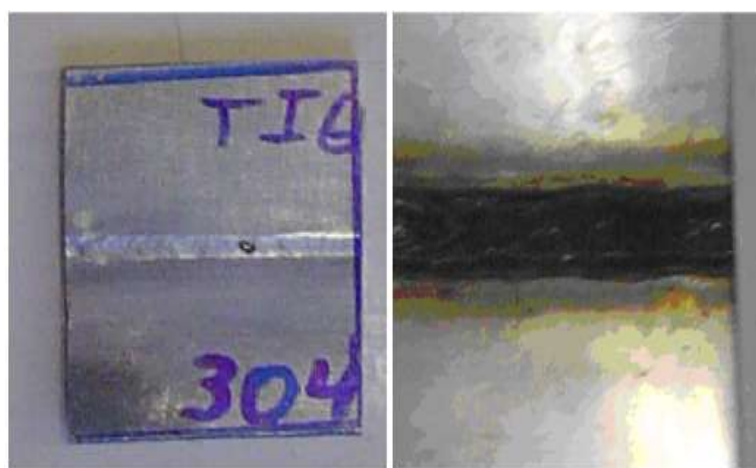
Figure 3. Aspects of the weld in TIG and MIG steels AISI 304.
